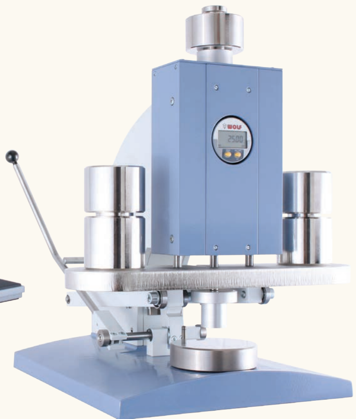
Thickness gauge on the basis of DM 2000 with contact apparatus especially for the testing of geotextiles and geosynthetics; via weights, the thickness can be measured under different specified pressures according to EN ISO 9863-1:2005. The image shows the device with additional weights for the measuring pressure 200 kPa
